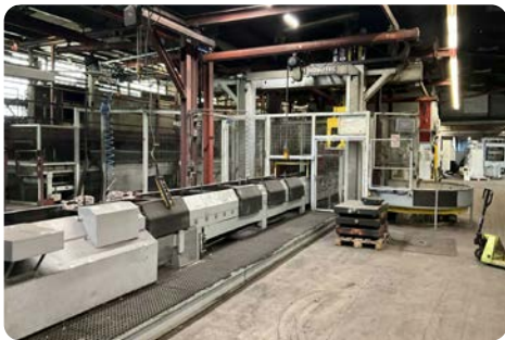
CNC controlled MOULDING LINE “Georg Fisher” Impact Standard IM-S1 (1988 – 2015) consisting of 1 forming machines, cap. 180 forms/h, each 20 seconds, mould dim. 900 x 700 x 300/300 mm.
