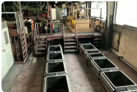
CNC controlled MOULDING LINE “Georg Fisher” Impact Standard IM-S1 (1988 – 2015) consisting of 1 forming machines, cap. 180 forms/h, each 20 seconds, mould dim. 900 x 700 x 300/300 mm.
